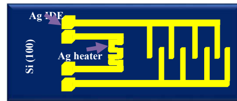
Ag sputtered IDE on Si substrate
